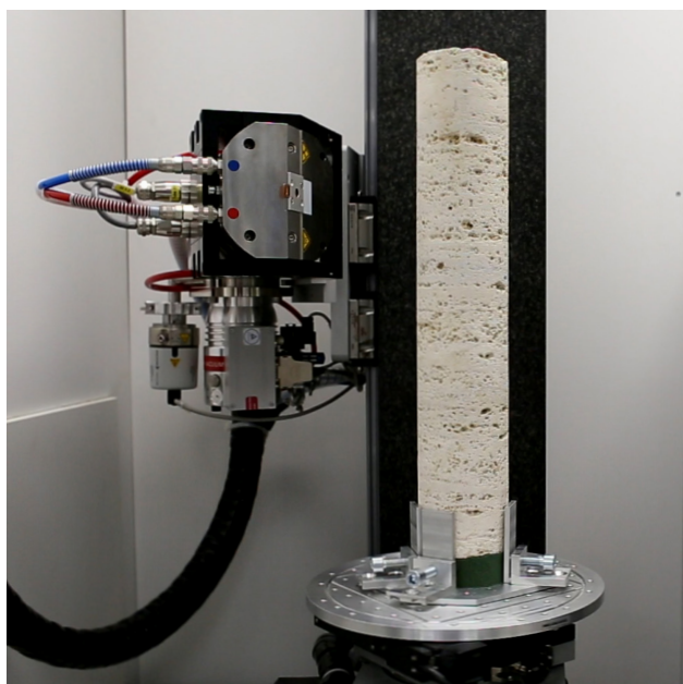
▲ Fig. 4: Interior view of TESCAN CoreTOM, showing a mounted rock specimen.
